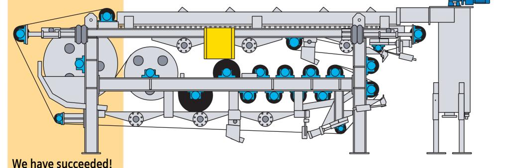
The mechanical stress over the rolls is reduced to a minimum by sizing them to a deflection below 0.6 mm/m at the middle of the roll. This is with a continuous operation with 9 kg/cm linear tension on the belts,
